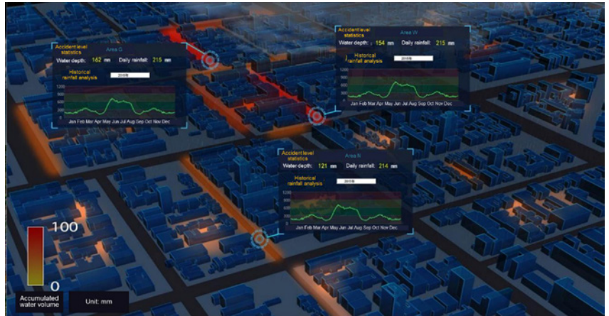
Figure 8 - Releasing warning information of urban waterlogging risks, based on real-time and historical data such as meteorological and water utilities data
