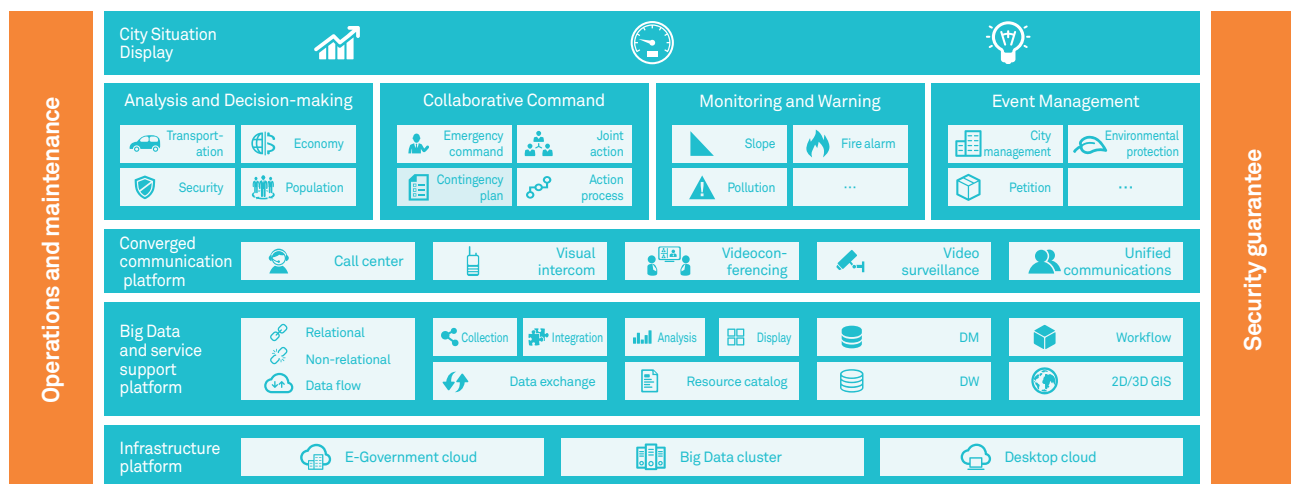
Figure 1 - Overall architecture of the IOC solution
